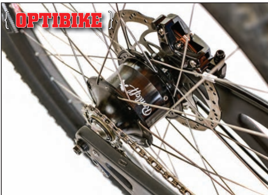
The Rohloff 14-speed, internally shifting rear hub is bulletproof and able to handle the extreme forces this bike can put on it. However, we found that it won't shift under load, even if it's just leg power.
