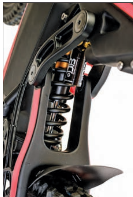
The ample Fox Float DPX2 coil-over shock is really good and well protected inside the frame.
