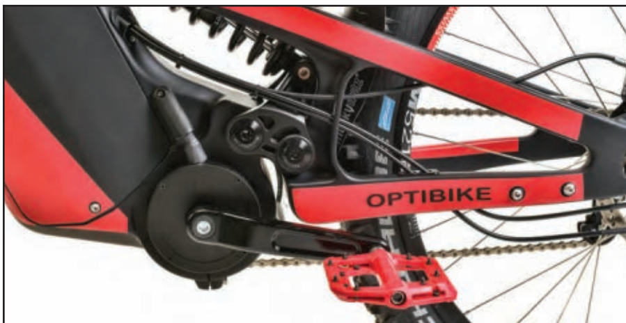
A closer look at the rear triangle and bottom bracket shows how compact this motor is for all its power, the suspension linkage and clever cable routing.
